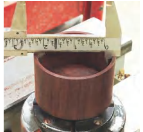
STEP 12. Measure the inside diameter of the box as you will need to transfer this to the apple. This is best done with a pair of Vernier callipers
